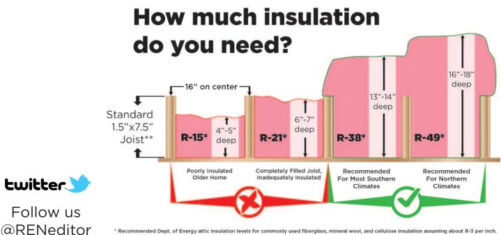
Recommended Dept. of Energy attic insulation levels for commonly used fiberglass, mineral wool, and cellulose insulation assuming about R-3 per inch. Standard joists are sold as 2"x8" but usually measure closer to 1.5"x7.5
